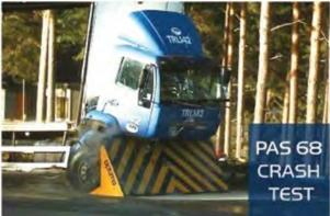
Optima HRR-HS-CT road blockers are crash tested and certified PAS68:
